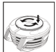
fig. 11 - fit side plate
